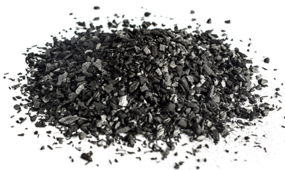
Granular Activated Carbon (GAC)
