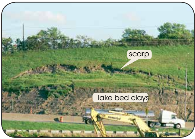
Figure 22. Long headscarp of a rotational slide in lake bed clays along I-75 in Hamilton County, Ohio. This was also the route of the old Miami and Erie Canal, whose aqueduct across Mitchell Avenue collapsed, likely due to lake clays.
