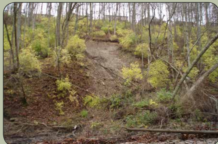
Figure 6. A small translational slide with debris pile at toe. Note the disoriented trees and exposed underlying bedrock of the Kope Formation.
