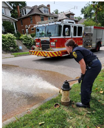
Exhibit 4: CFD Firefighter flowing a fire hydrant. Company Engine 46 also pictured.
