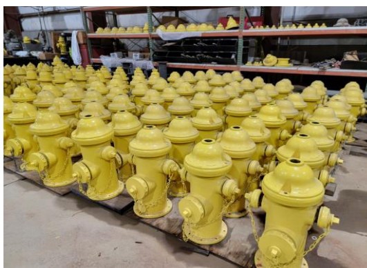
Exhibit 2: Fire hydrants stored at GCWW following reconditioning.
