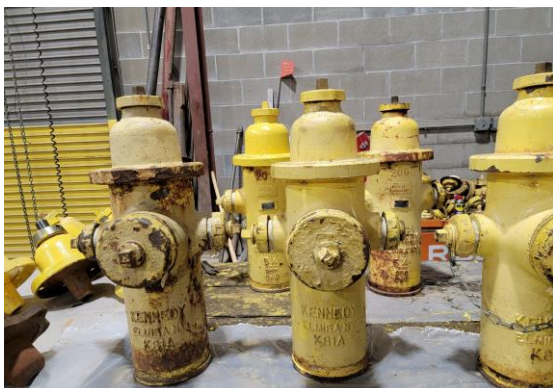
Exhibit 1: Fire hydrants ready to be repaired, painted, and tested at GCWW.
